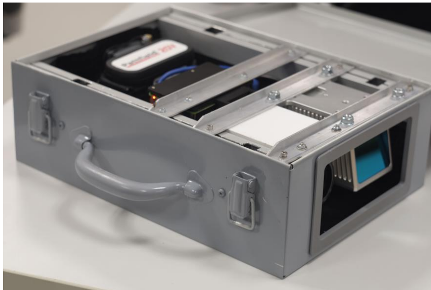
Fig. 1 Internal configuration of the logger unit
