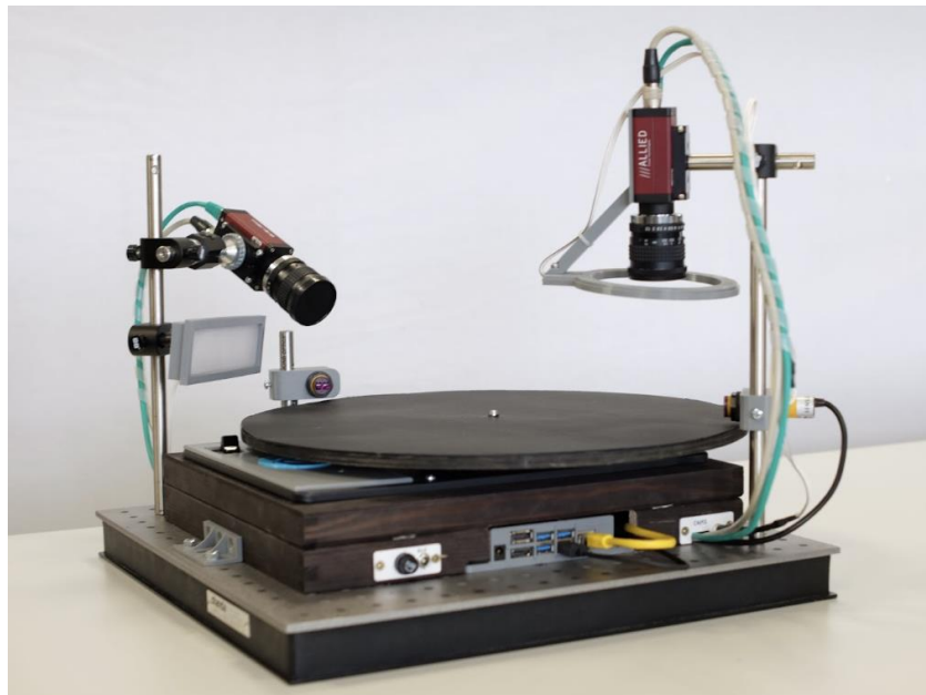
Fig. 3. Overall view of the demonstration platform for anomaly detection with no connections, no task-specific base and no inspected samples – core structure
