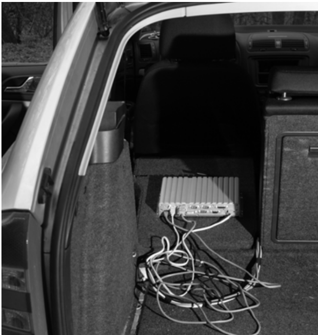
Fig. 7. Placement of the VTC6100 vehicle telematics computer in the luggage compartment.
