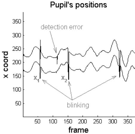
**Fig. 11.** The recognition between errors and moments with closed eyes
