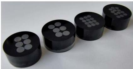
Fig. 1. Examples of the six-wired and the twelve-wired cylinders.
