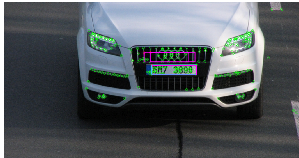
Fig. 7. SURF interesting points (green circles) detected in a sample image and potential license plate regions (violet rectangles).
