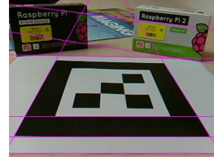
Figure 7. Eight lines related to the eight strongest peaks in the accumulator in the Fig. 6 imprinted into the input image.
