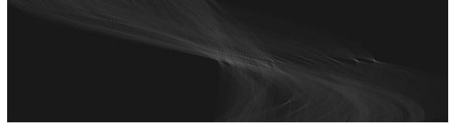
Figure 6. The accumulator of the Hough transform in form of a grayscale image containing several peaks representing respective number of lines in the input image.
