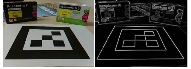
Figure 3. The input RGB image from RPiCam with resolution of 320x240 pixels and the relevant result of the Sobel operator.
